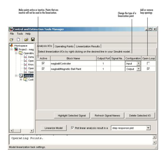
**Note** You cannot make changes to the **Analysis I/Os** or perform open-loop analysis when you select Numerical Perturbation as the **Linearization Algorithm** in the Linearization Task Options window (accessed by selecting **Tools > Options** from the Control and Estimation Tools Manager window). See "Changing Linearization Settings" in the online Simulink Control Design User's Guide for information.
