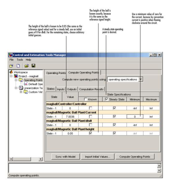
When you add states, inputs, or outputs to the model, or remove them from the model, click the **Sync with Model** button to update the operating point table to reflect these changes.
