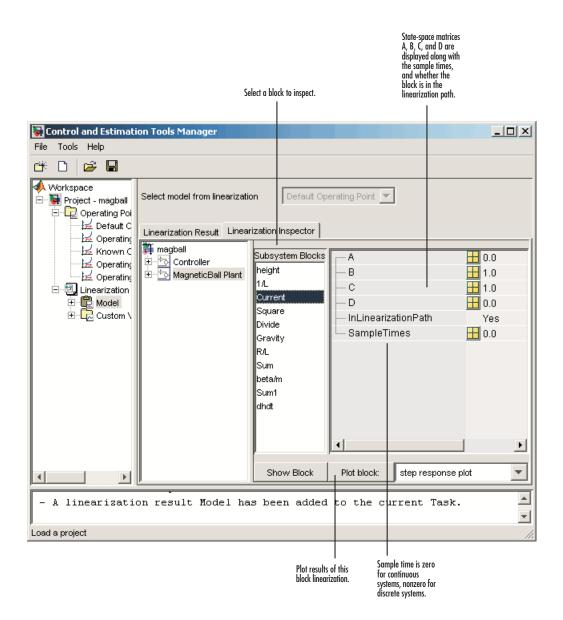
**Note** The **Linearization Inspector** pane does not exist for models that are linearized with numerical-perturbation linearization (when Numerical perturbation is selected as the **Linearization Algorithm** parameter in the Linearization Task Options window) as there are no individual block linearizations to inspect.
