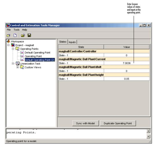
**4** Edit the operating point by entering new values in the table. Switch between state and input values using the tabs on the left.
