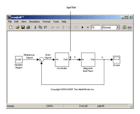
3 Right-click the signal line after the Magnetic Ball Plant and select Linearization Points > Output Point from the menu.
