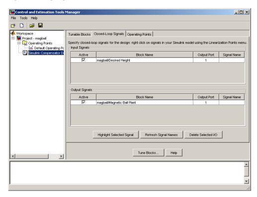
Within this pane you can view the input and output signals in the model and use the **Active** column to select the ones you want use to define closed-loop systems for compensator design.
