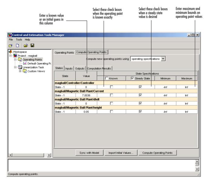
**3** Enter operating point specifications in the table, such as any known values or constraints on signal values. Switch between states, inputs, and outputs using the tabs on the left.
