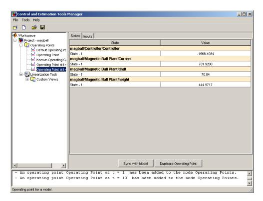
When you add states, inputs, or outputs to the model, or remove them from the model, click the Sync with Model button to update the operating point table to reflect these changes.
